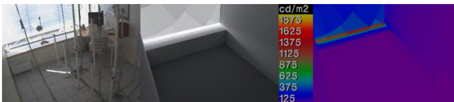
Figure 18: Photo of the experiment room at 09.30, 23.07.2014 and rendering from Radiance showing that the light stripe penetrating into the room is not detected in the simulation.
