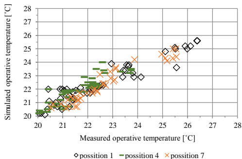
Figure 13: Comparison of simulated T_{\text{op}}^S with the new zone model in IDA ICE and measured T_{\text{op}}^S for position 1, 4 and 7. Total observations n=147 , correlation coefficient R=0.95 (position 1), R=0.89 (position 4) and R=0.96 (position 7).
