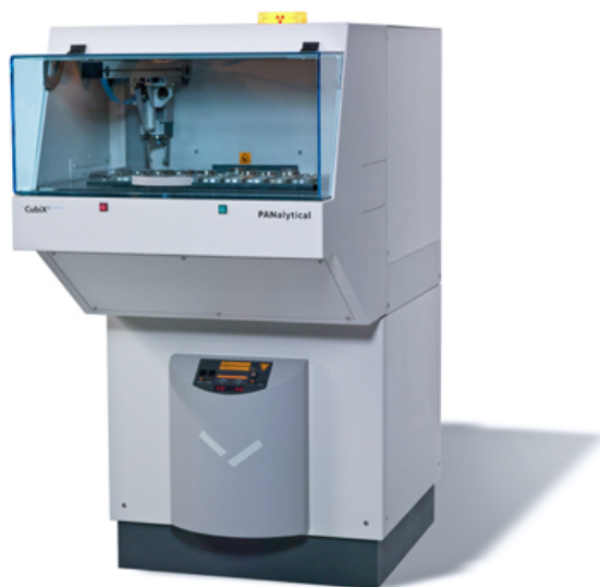
FIGURE 4.10: The PANalytical CubiX PRO X-ray diffractometer used in this study.
