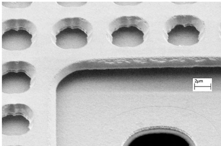
Fig. 4. Scanning electron micrograph of a ventilation hole in the membrane, exposed in a larger opening in the perforated back plate.
