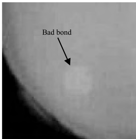
FIGURE 8. IR picture of one quarter of the 4 inch fusion bonded wafer where a disbond is observed.
