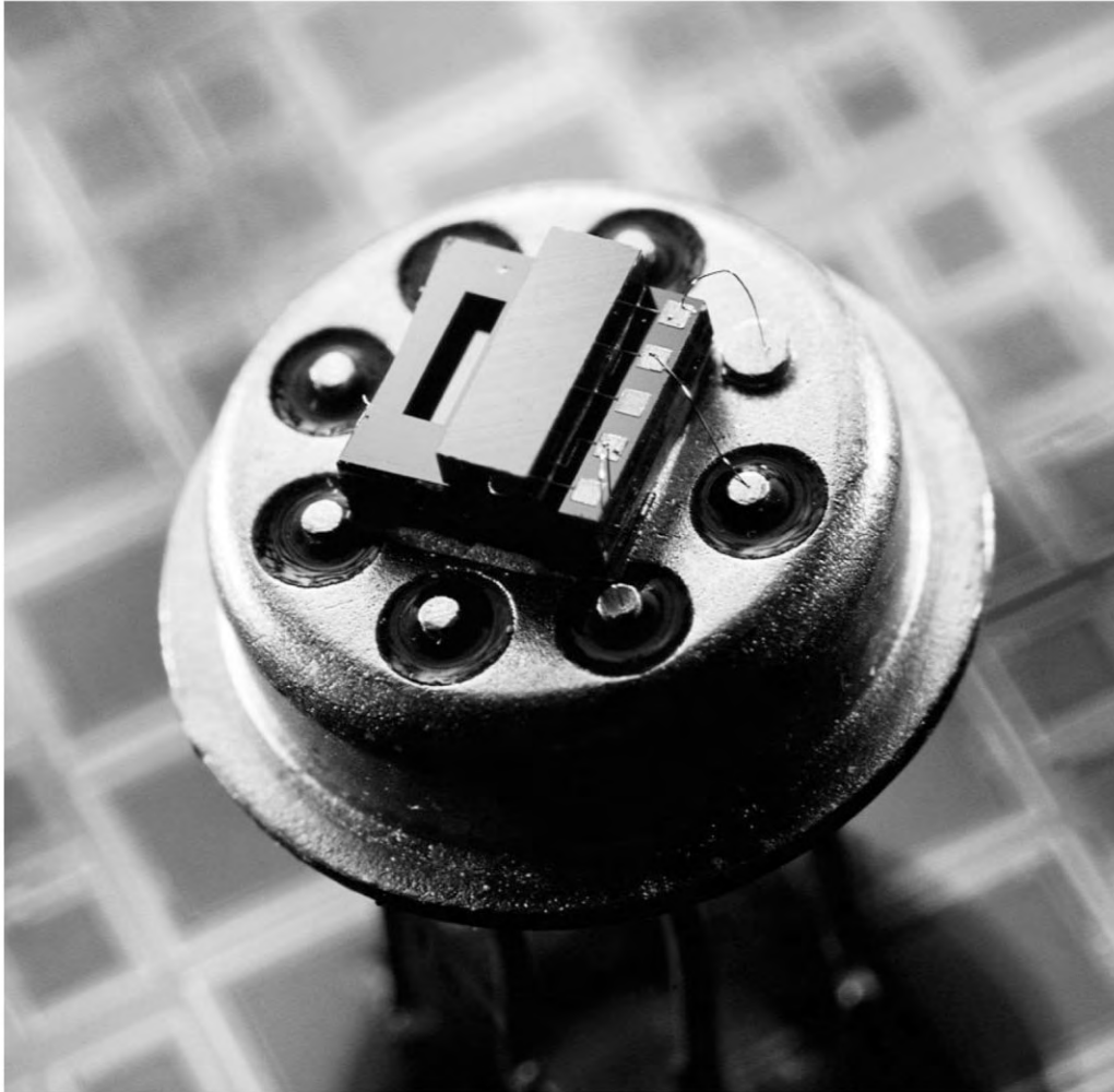
Fig. 6. Complete silicon microphone stack mounted in a TO5 housing for testing. Further processing includes the polymer coating and flip-chip mounting of a flexible printed circuit board and a sound inlet.
