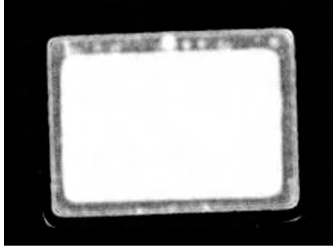
FIGURE 15. C-SAM picture of lid solder interface of package housing (approx. 8 mm · 4 mm · 3 mm) for MEMS and microelectronics. White areas in soldered rim are without contact between lid and solder.
