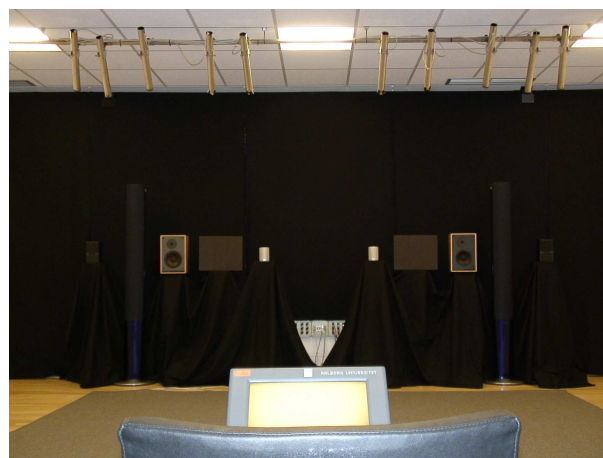
Fig. 7: Photograph of the setup (room fully illuminated). The fake wall is covered with a black cloth. The spot lights that illuminate the loudspeakers during the experiment are also visible. In the foreground, the chair for the subject and the touch screen are shown. The loudspeaker cable connections were left visible for the sake of plausibility.
