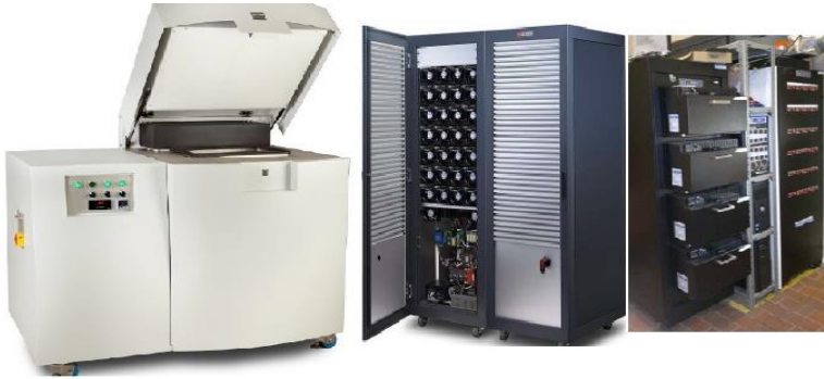
Figure 6 Experimental Framework Measurement Tools. [Left]Netzsch® Isothermal Calorimeter [middle]Digatron® Battery tester, [Right] Maccor® Battery Cycler.
