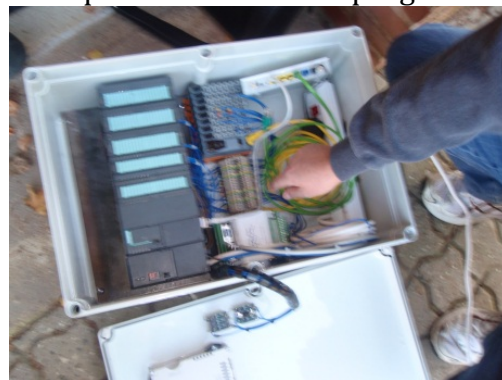
Figure 7.8: The suitcase containing the Siemens PLC and interface-modules. Picture by Author, fall 2011.
