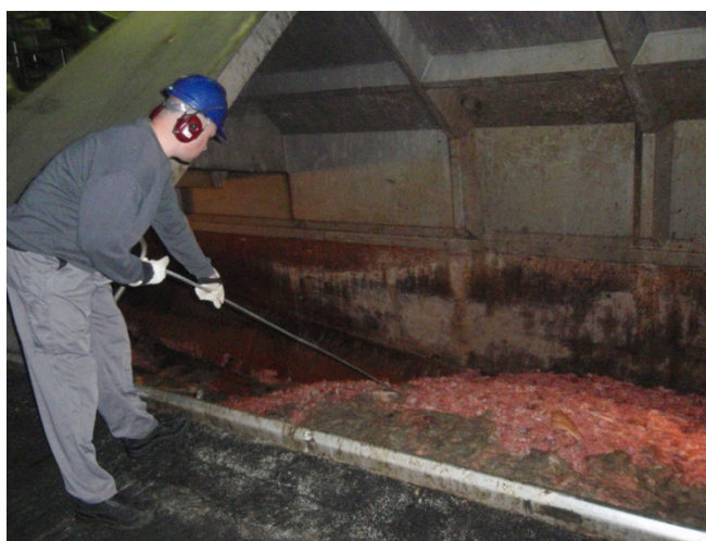
Figure 5.7: Own photo of a raw product container. An operator is seen while trying to remove a misplaced plastic box that came with the raw product.
