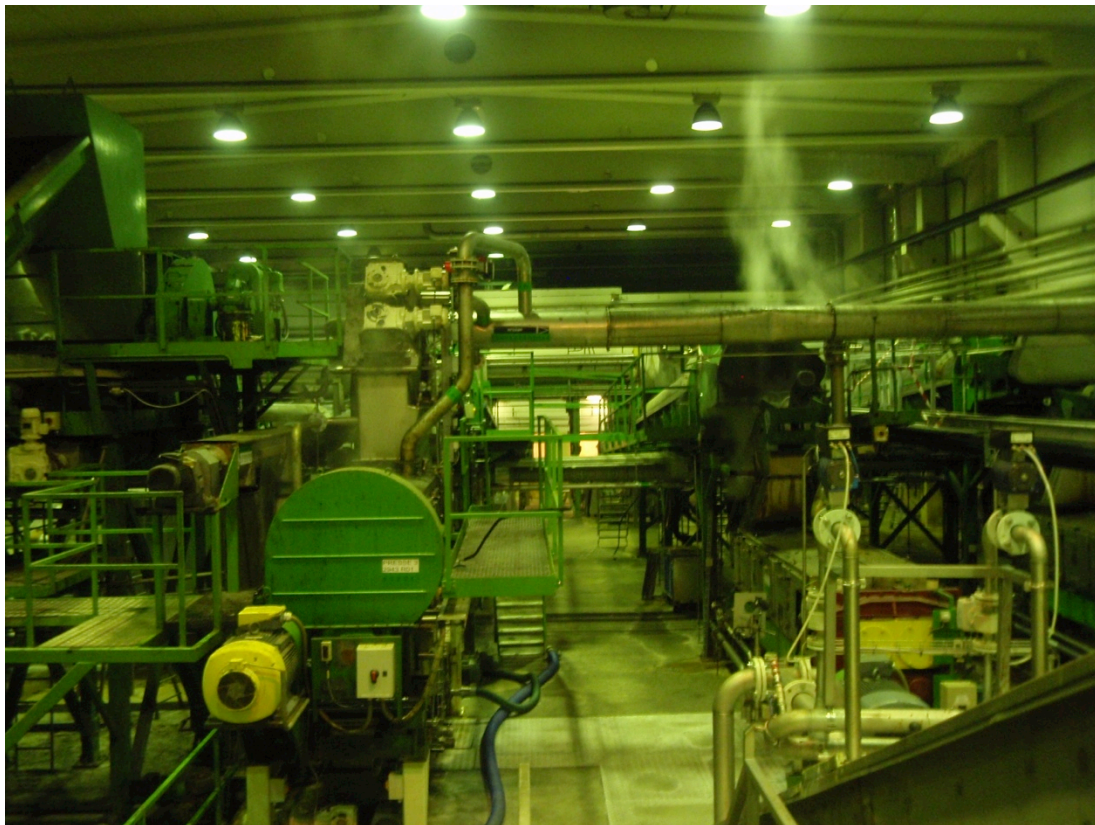
Figure 5.8: Picture taken by author during 2011 of the factory fall housing the press-lines with the mincers, the thermo-screws and press machines.
