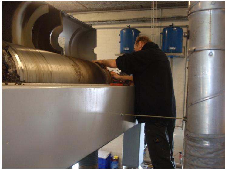
Figure 7.6: The decanter expert has opened the decanter to check its sensors and clean it. Picture by Author, fall 2011.
