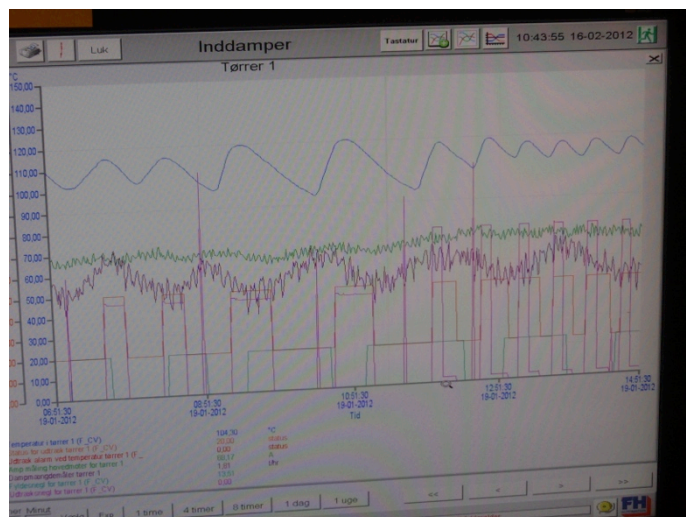
Figure 6.9: Temperature variations with and without the new "out of phase" steering. The left part of the plot shows the operation caused by the basic steering. The right part of the plot shows the effect of the new steering scheme. Picture taken by Author, fall 2011.
