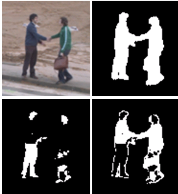
Figure 6.4: Top-left: the input image. Top-right: the foreground mask F . Bottom-left: the pixels classified by the upper-leg appearance model C . Bottom-right: the mask that is searched for possible occluded upper legs O , i.e. the foreground mask except the mask from the appearance classification.
