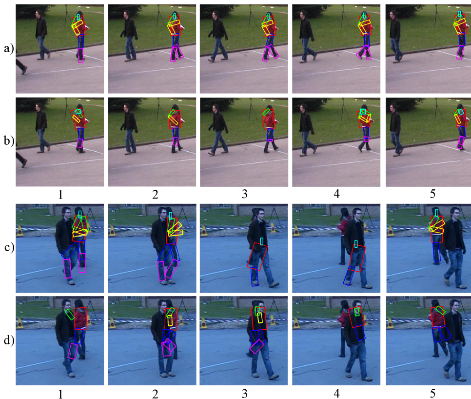
Figure 7.4: Comparison of the multi-view approach against the single-view approach. Rows a) and c) show the results of pose estimation with the single-view approach. Rows b) and d) show the results of pose estimation with the multi-view approach. Each column of the figure shows a frame from two synchronized cameras.
