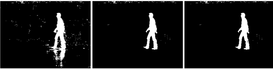
Figure 5.16: Three segmentation results with varying values of \sigma . Left: \sigma -value too low. Middle: optimal \sigma -value. Right: \sigma -value too high.
