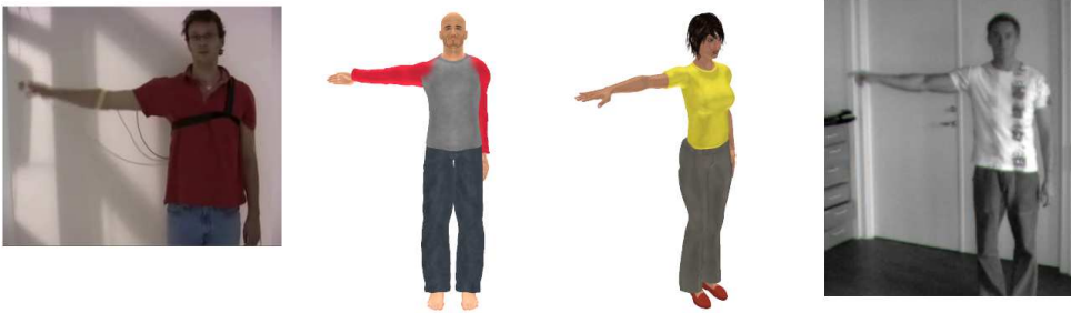
Figure 3.6: An illustration of the different types of data used in the system. From left to right: 1) 3D tracker data is acquired from magnetic trackers mounted on persons who perform the five actions. 2) The tracker data is animated in Poser from a fronto-parallel view. 3) The tracker data can be animated from any view point with different clothings and models. 4) After training the primitives on semi-sythetic data we recognize actions in real video.
