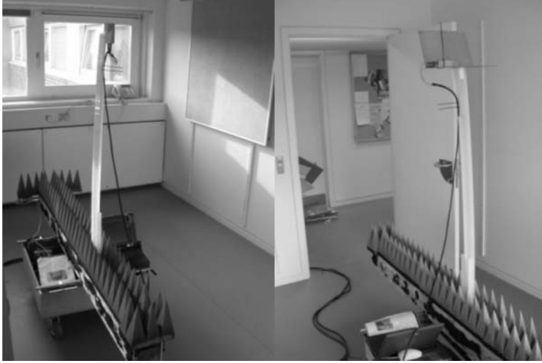
Figure 2. Orientation of the handset and laptop in the measurement campaign
