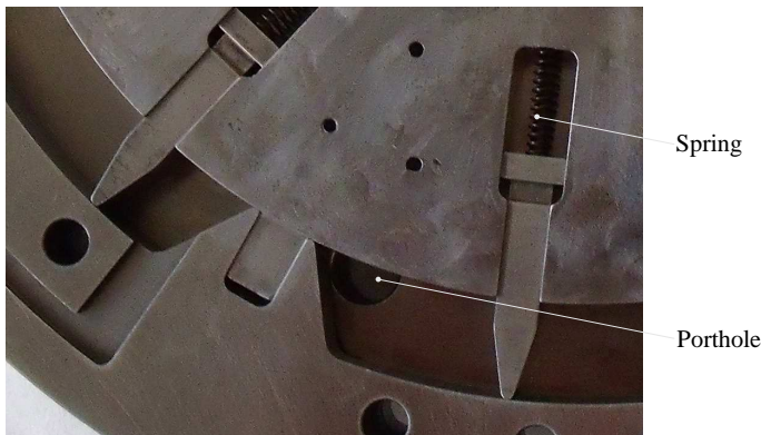
Figure 2.10: A porthole through the inner and outer housing is useful for a visual inspection of the movement of the vanes.
