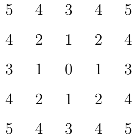
Figure 1.2: The zeroth- to fifth-order neighbours of the middle site in a five times five regular square lattice.
