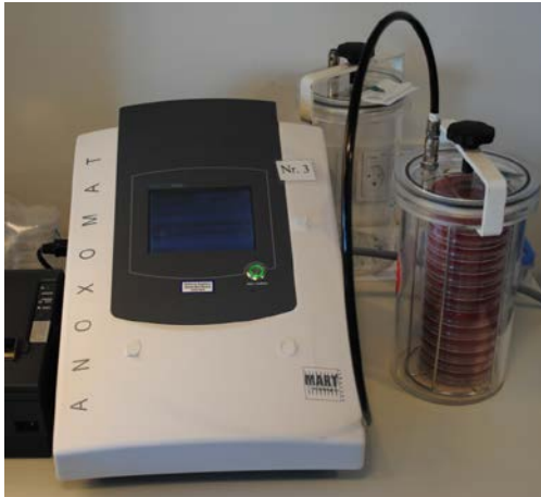
Figure 5: The Anoxomat Mart II chamber system. Used for implementing different incubation environments. (Author's own photo).
