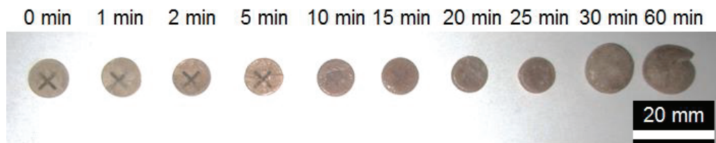
Figure 3. Photographs of the as-prepared MOF glasses for different melting durations. The samples with “X” were used to assess the variation in the transparency by using naked eyes.
