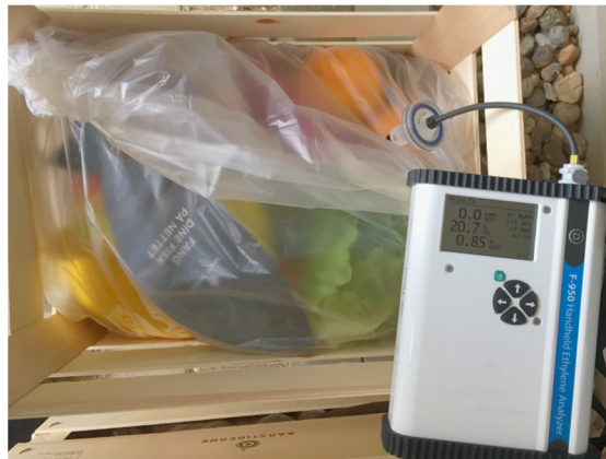
Figure 3-5 Bag of mixed fresh produce and sensor used to record the generated C_2H_4 levels.
