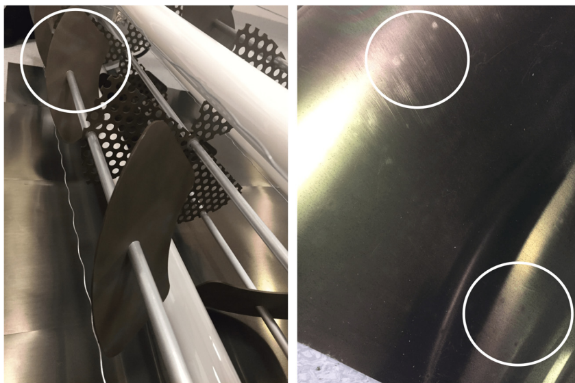
Figure 5-16 TiO_2 -coated surfaces showing signs of deactivation through oxidation patches (left) and spots (right).
