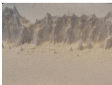
Figure 4. Solution 5 electrospun with a 1D needle movement. The structure is seen to be self-supporting.
