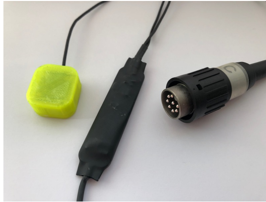
Fig. 4.1: Example of one of the accelerometers used in the studies (yellow plastic housing), the power supply, filter and amplifier sleeved in black and the DIN8 plug.
