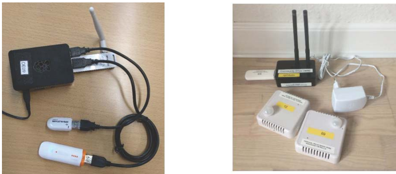
Fig. 5.6: RaspberryPi and Environmental Sensors
