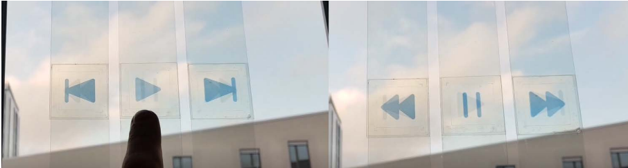
Fig. A.13: Application examples. Touch sensitive transparent buttons mounted on a window.
