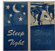
Fig. D.5: Example of electrochromic display. Left : Side A visible. Right : Side B visible. The bright parts let light through and thereby projects intricate shadows.
