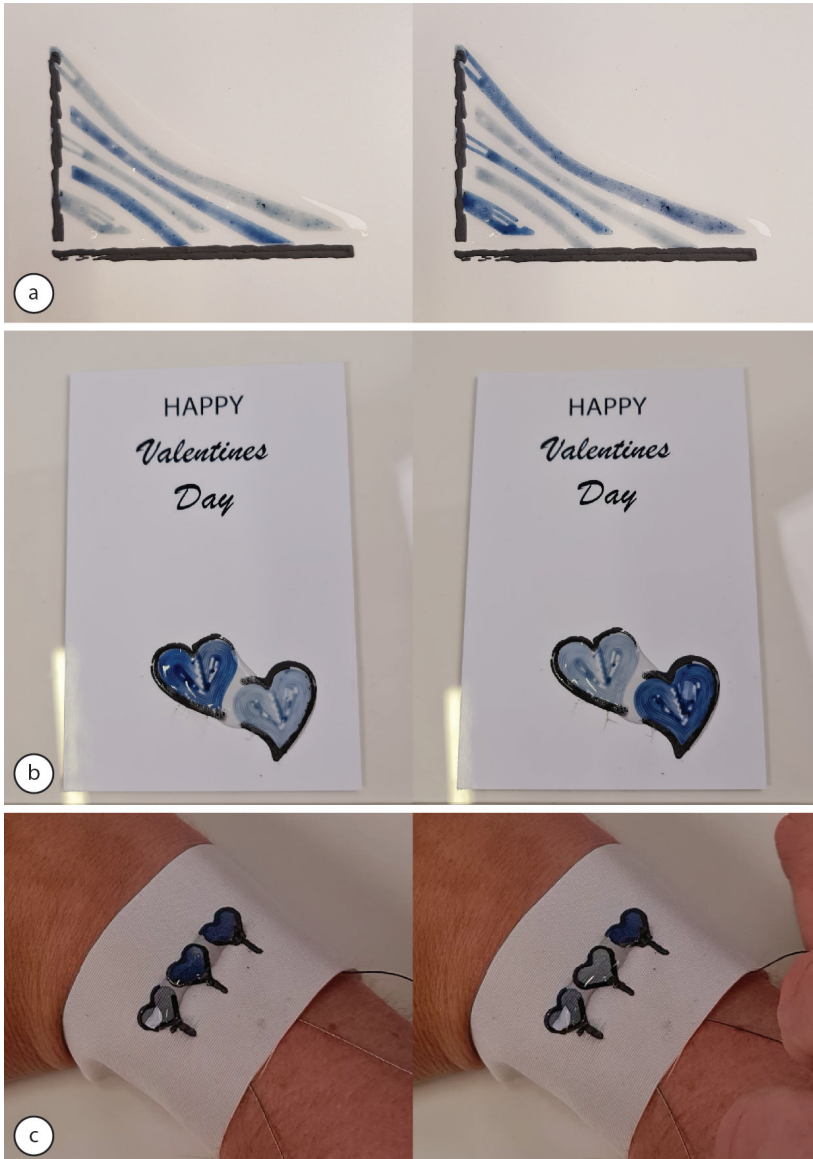
Fig. B.7: Functional prototypes printed using ECPlotter: (a) a display printed on ceramic tile, (b) a display printed directly on photo paper and (c) a display printed on polyester fabric.
