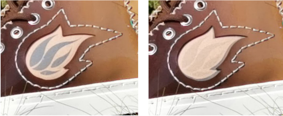
Fig. F.1: Raised heart rate indication in activated and deactivated states.
