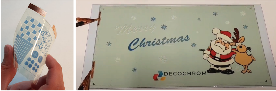
Fig. 1.1: Examples of electrochromic devices. Left example shows the flexibility of the technology (Paper A) [8]. Right example shows how the transparency of electrochromic devices can work in combination with traditionally printed graphics. The snowflakes and text is part of the electrochromic device whereas the Santa, reindeer and DecoChrom logo is inkjet printed on normal paper and placed underneath.
