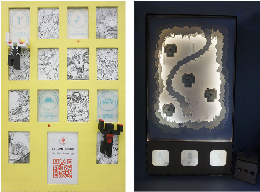
Fig. C.4: Left: The Spider-Man artifact features a building facade with multiple ECDs and two movable, 3D-printed characters. Right: The Centipede artifact is the physical representation of the 2D game with mushroom-shaped electrochromic displays taking the form of shootable objects. A laser-cut controller selects which character is activated.
