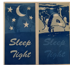
Fig. D.5: Example of electrochromic display. Left : Side A visible. Right : Side B visible. The bright parts let light through and thereby projects intricate shadows.
