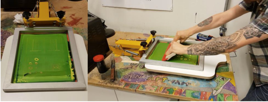
Fig. 3.3: Left: Frame with negative stencil. Right: Squeegee being moved across the frame pressing ink through the exposed parts. (Part II, Paper A) [22]
