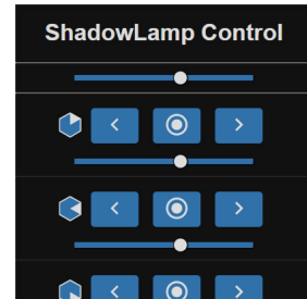
Fig. D.6: Part of the ShadowLamp Control User Interface. Sliders control brightness of LEDs and buttons control which side is visible with middle button making neither side visible
