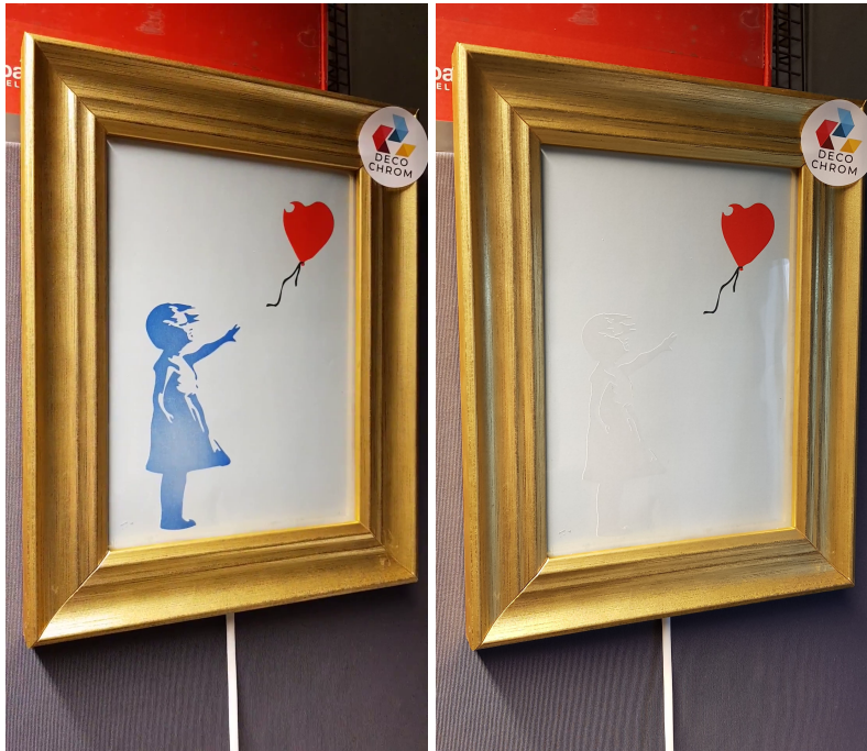
Fig. 4.2: Electrochromic Art Piece example of Banksy's Girl with Balloon . The girl is created with electrochromic display technology whereas the background and the balloon is printed using traditional ink-jet printing. The electrochromic display is overlaid the traditional print allowing the girl to appear as one with the background and disappear instead of being shredded.
