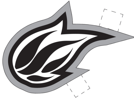
Fig. F7: The electrochromic display design, showing counter electrode (black bar around flames), border areas (grey) and connection areas (dashed).
