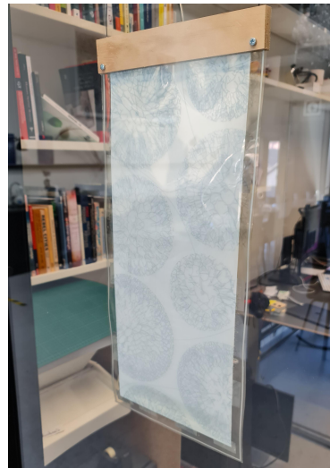
Fig. 4.1: Example of wallpaper type electrochromic display. Fabricated by Ynvisible (DecoChrom partner).
