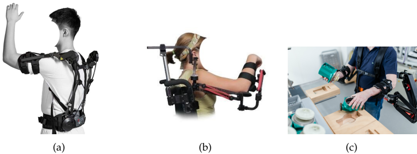
Fig. 1.5: Examples of passive upper body exoskeletons; (a) CDYS [41] (b) WREX [39] (c) ROBO-MATE [42]
