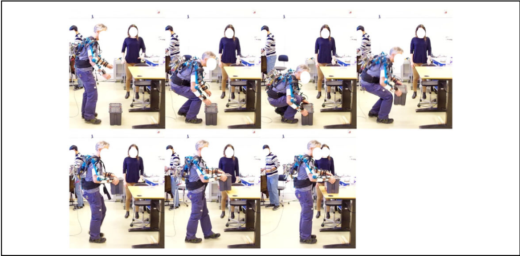
Figure 14. Test of the UB-AXO with 6 kg payload lifted from the ground to a table.
