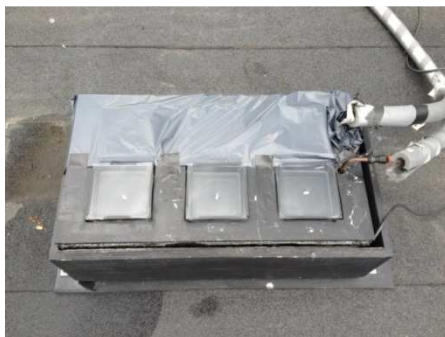
Picture 3-2 Outdoors photodegradation study setup.
