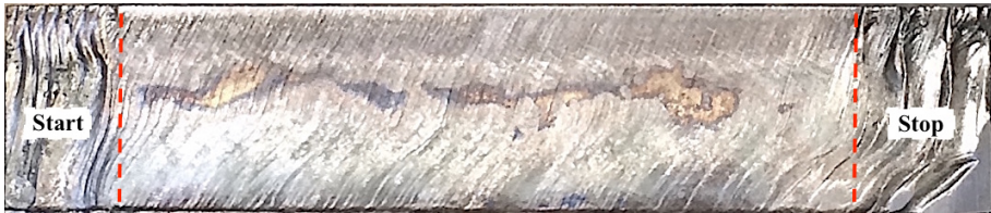
Fig. 4.4: Surface appearance of oxygen assisted laser cuts: 680\ \text{mm}/\text{min} travel speed and 3 kW laser power (120 mm length).
