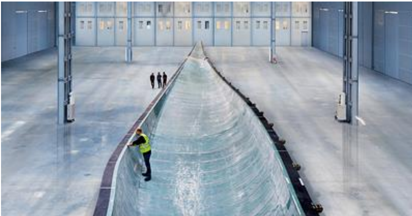
Figure 28: Mould for Siemens 75 meter blade (2012).
