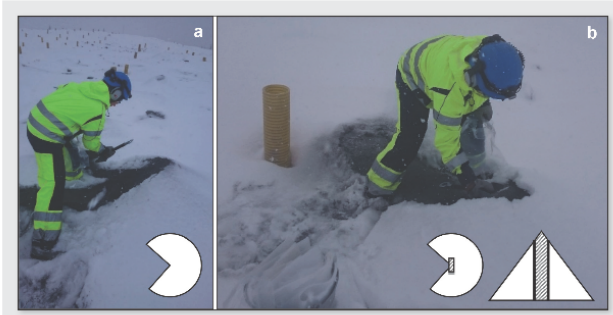
Figure 2. Manual BH sampling at a LKAB open pit mine. a. Cutting a section of the BH core. b. Collecting a vertical slice of uniform thickness from the bottom to the top in the centre of the blast hole core.
