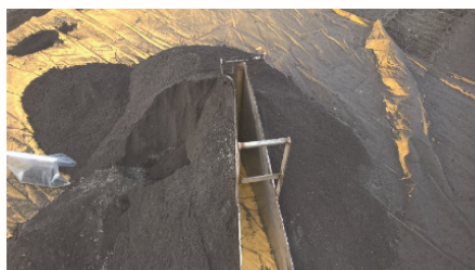
FIG 7 – Manual and segment sample collected from a coarse blasthole cone.
