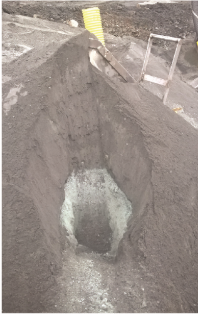
FIG 3 – Blasthole cone originating from drill hole with large variations in iron grade at different depths of the drill hole. The white material is rich in silica, while the black material is rich in iron. See text for a detailed geology description of the Leveäniemi ore and gangue.
