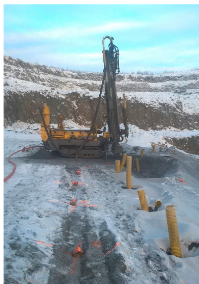
Figure 4. Explorac 100 RC drill rig in action during the twin hole drill sampling experiment (winter in northern Sweden). The tubes mark the Blast Holes transect whereas the exposed rocks mark the twin RC holes.
