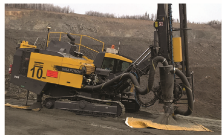
FIG 5 – Experimental drilling with canvas placed under the back discharge and canvas plus sectorial cutter placed under front discharge of the Atlas Copco D65 drill rig.
