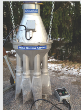
Figure 8. Top: Drillsampler™ from Harrison Cooper for automatic blast hole sampling installed underneath the drill deck (reproduced from Reference 2 with permission). Bottom: the Finnish "Autosampler" system with Soltforce™ sample socks attached (reproduced from Reference 24 with permission).
