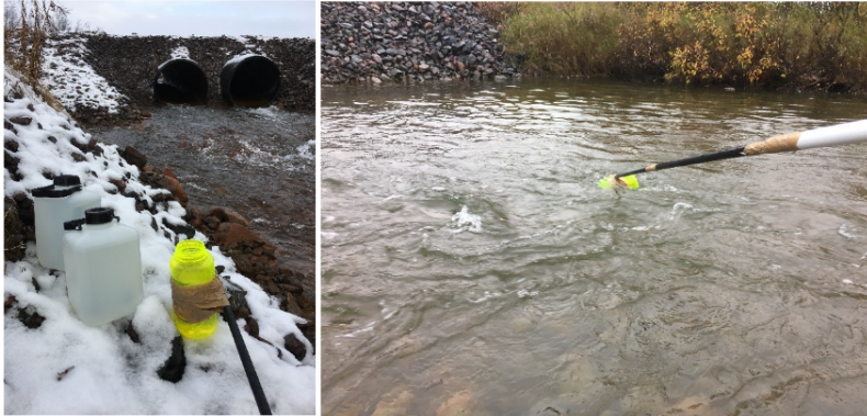
Fig. 2 Extendable pole with standard plastic sample container used to collect water samples according to the official protocols in the present study
