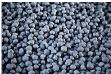
Figure 3. LKAB iron ore pellets for direct reduction steel making (photo: Fredric Alm)
