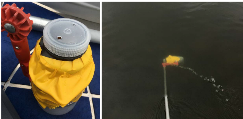
Fig. 3 The Aloha Sampler™ designed for composite sampling, for example along a complete cross section of the streaming water
