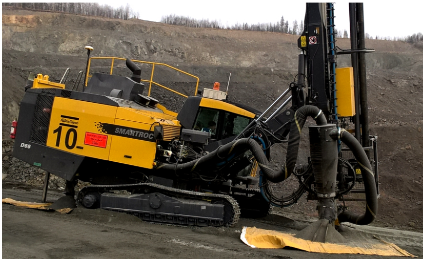
Figure 14. BH drilling and sampling using a stationary radial bucket, during one of the variographic experiments conducted within this Ph.D. study. The pictured D65 drill rig utilises a cyclone to separate fines and dust to a separate BH cone in the back of the drill rig.
