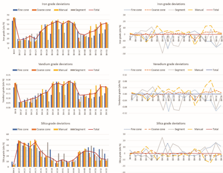
FIG 10 – Comparison of iron, silica and vanadium grade from 18 completely sampled blastholes to evaluate deviations for manual and segment samples in regards to the authoritative reference (the total weighted average from all collected material for each hole).
