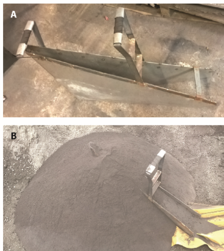
FIG 6 – (A) Sectorial sample cutter for delimitation and extraction of 'segment samples'. (B) Sectorial segment cutter at work in a typical blasthole coarse particles cone. A canvas is placed under the cutter to separate the blasthole material from the pre-existing ground material.
