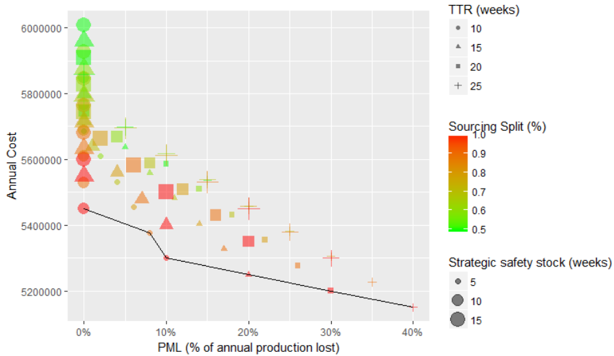
Figure 5.9: A Pareto frontier for alternative supply chain designs reflecting supply chain vulnerability (PML) and annual cost
