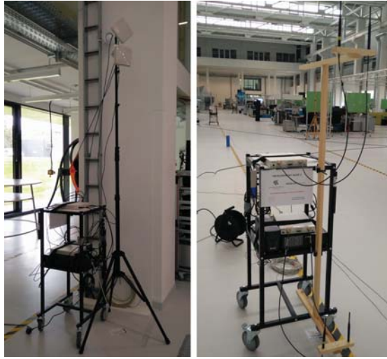
Fig. G.3: Nodes of the SDR testbed. The left image shows a transmitter node and the right image a receiver node.
