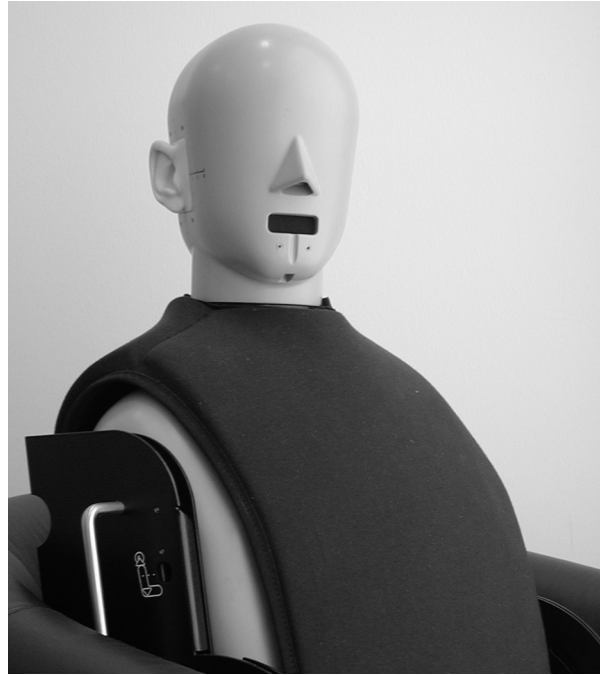
Figure 16: A head and torso simulator with the possibility of head rotation through a motor controller.
