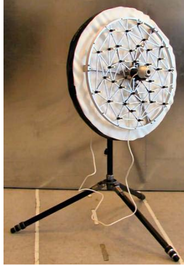
Figure 6: A planar array with a back screen. The array consists of 36 microphones.
