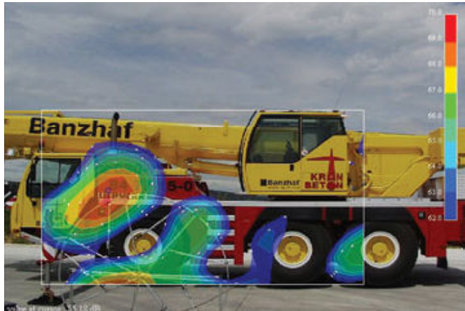
Figure 13: An example of beamforming applications to a large object, i.e. crane in this case, from a distance. The picture was taken from Christensen and Hald (2004).
