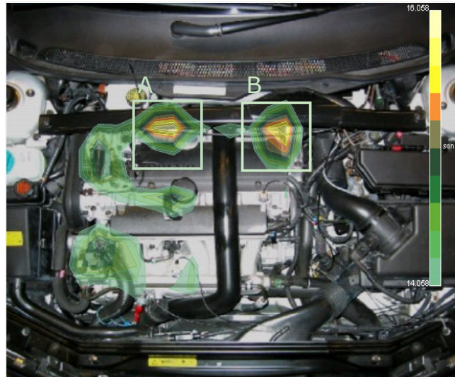
Figure 14: The loudness map of an engine compartment demonstrating that there are two noise sources having an almost identical size and peak loudness value.
