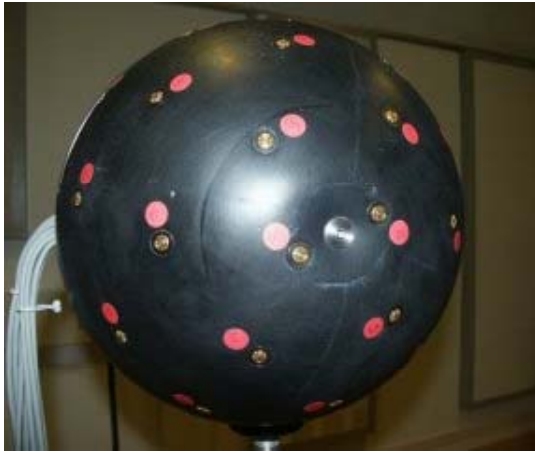
FIG. 5. The array consisting of 64 microphones placed on the hard surface of a sphere having a 14-cm radius. The dots on the sphere indicate the microphone positions.
