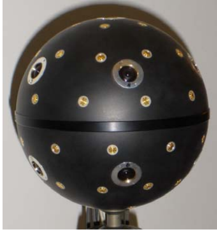
Figure 5: A spherical array with 50 microphones and 11 small cameras mounted flush on a rigid spherical surface with a diameter of 19.5 cm.
