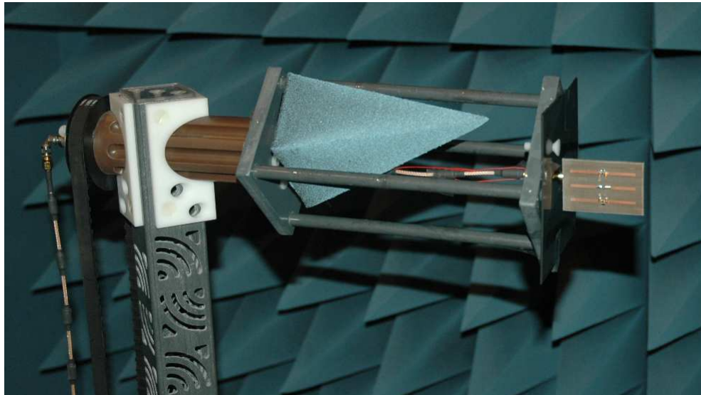
Figure 4.8: Set-up of the antenna for reconfigurable radiation pattern measurements, with a 9V battery placed behind the absorber cone in a direction of the low field intensity.
