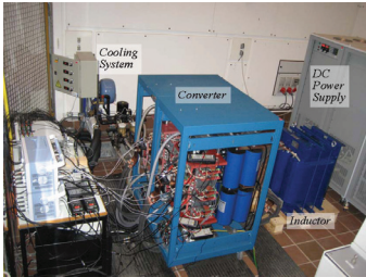
Fig. 8. Test setup photo
