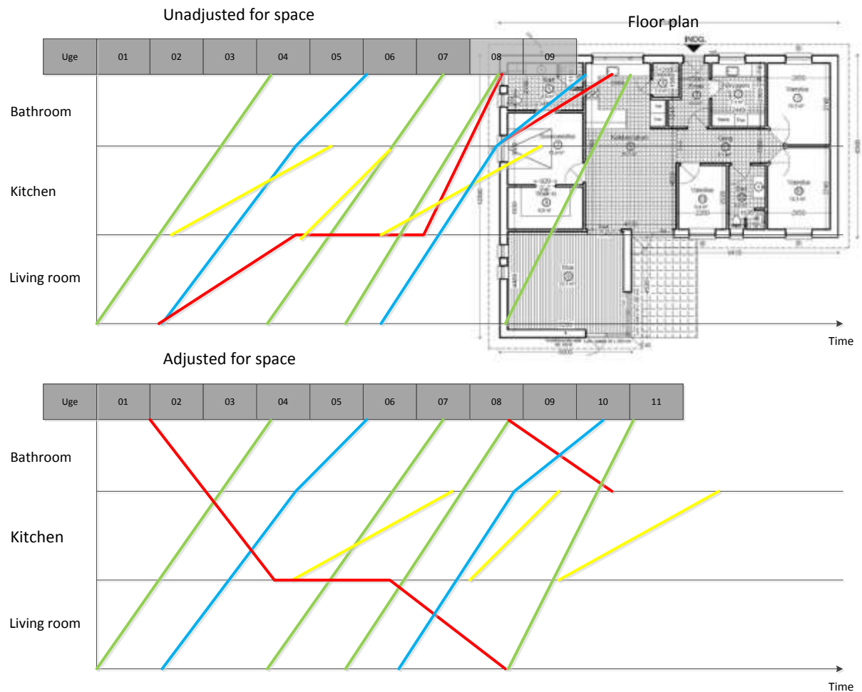
Figure 5: Example; adjusting for space usage. Applying a cyclogram and compare it to the floor plan to identify insufficient space and adjusting sub-sequences. The colors in the cyclogram represent the subcontractors on-site.
