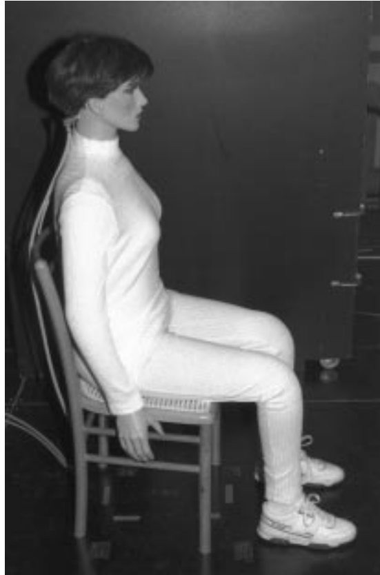
Figure 2.7. Breathing Thermal Manikin used to measure the personal exposure. The manikin is separated in 16 individual parts of the body, each with the same surface temperature and heat output as people in thermal comfort. The manikin has an artificial lung to simulate breathing. Height = 1.7 m, A_{Du} = 1.5 \text{ m}^2 , I_{cl} = 0.8 \text{ clo} .
