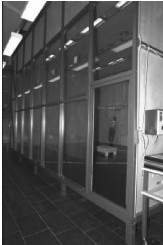
Figure 3.5. Photo of the full-scale test room with a floor area of 48 m 2 and a height of 4 m in the present set-up. On the photo the double glazing in one of the walls is seen, applied to facilitate smoke visualisation.
