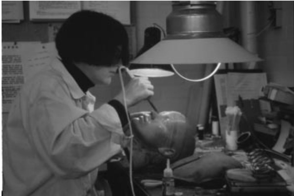
Figure 2.6. The Breathing Thermal Manikin under construction at the Technical University of Denmark. Here, the resistance wire used for heating, measuring and controlling the skin temperature and the heat output is mounted on the head.
