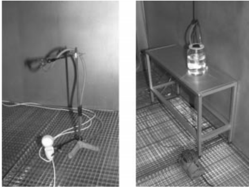
Figure 3.25. Photo of the Sensory and chemical contaminant source used in the present measurements (see Figure 3.24.). Left: 2-propanone delivered above a hot light bulb. Right: Passive evaporation of liquid 2-propanone.
