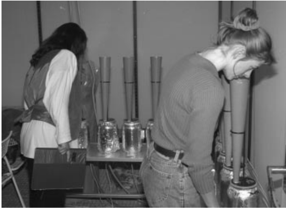
Figure 2.15. Members of a Trained Sensory Panel assessing the air quality in comparison with five levels of a known reference.
