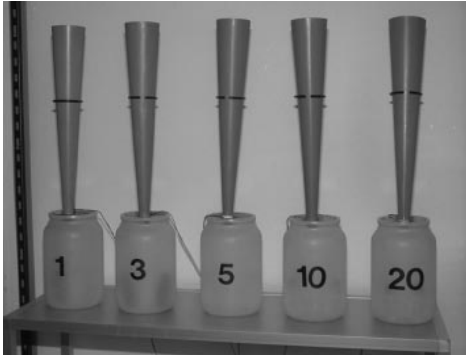
Figure 2.14. Five known 2-propanone references (milestones) of 1, 3, 5, 10 and 20 decipol used by the Trained Sensory Panel for judging the perceived air quality. The references consist of a 3-litre glass jar with a ventilated diffuser ( \sim 0.9 l/s). Inside the jar the 2-propanone is generated by passive evaporation from pure liquid 2-propanone in 30 ml bottles. According to Bluysen and Fanger (1991) the references can be calibrated using the relation: \text{decipol} = 0.84 + 0.22 \cdot \text{ppm} .
