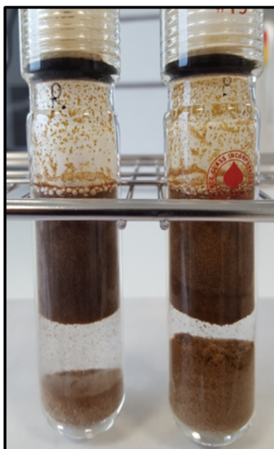
Fig. A1: The right hand side test tube showing the frequent shaking while the left hand side test tube showing the appropriate shaking (twice a day for few seconds) results.
