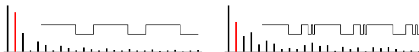
Figure 3.31: Spectra of PWM (left) and PCM (right) current shape. Base frequency, marked with red bar, is 200 Hz in both cases. The DC value for both signals is the same. The PCM signal contains more high frequency components in the spectrum.
