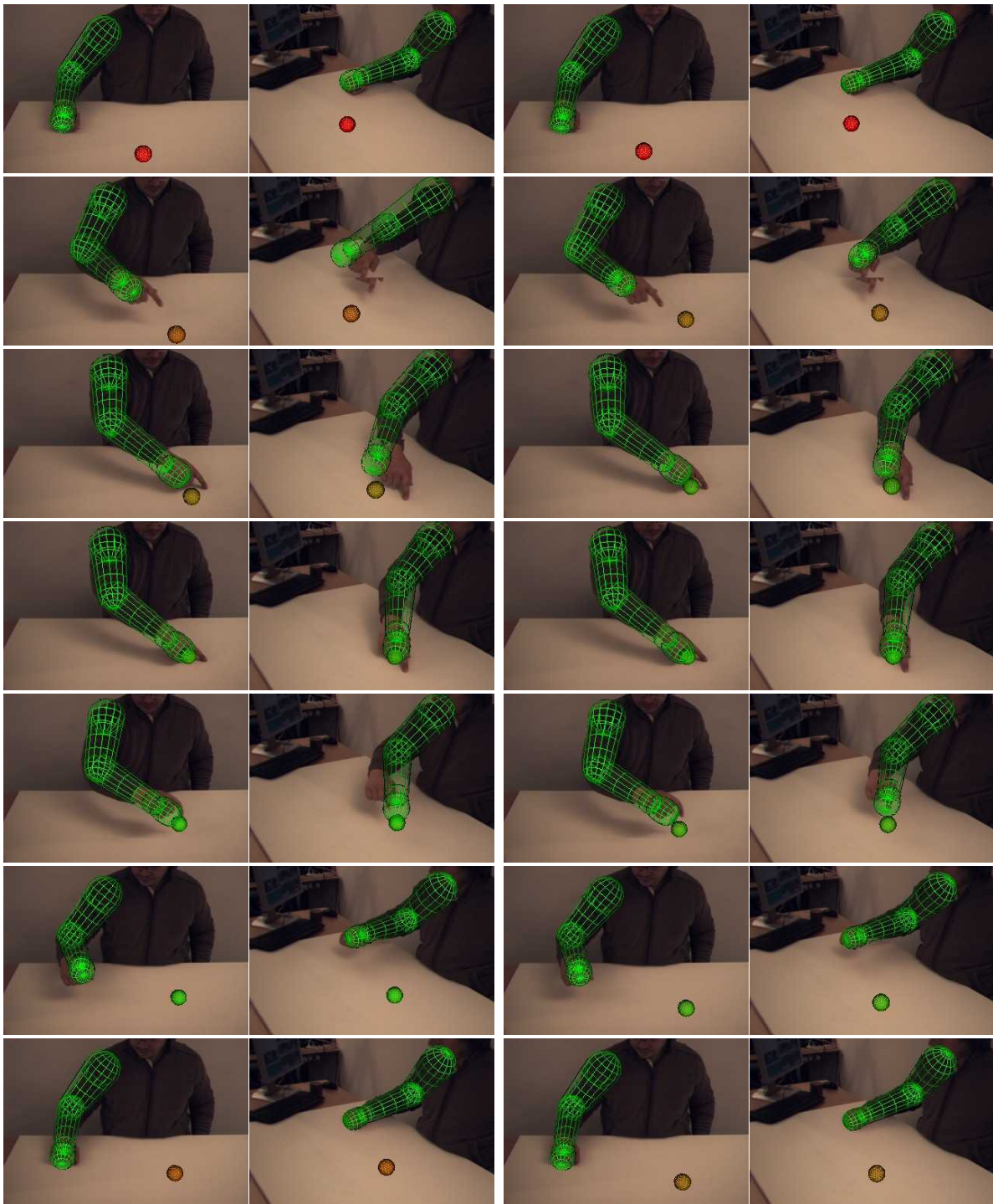
Figure 6.18: Pointing Trial 2. On the left, the camera views of the cameras 2 and 4 are shown, where only camera 2 is used for tracking. On the right, the same camera views are shown, where all cameras (1, 2, 3, and 4) are used for tracking.
