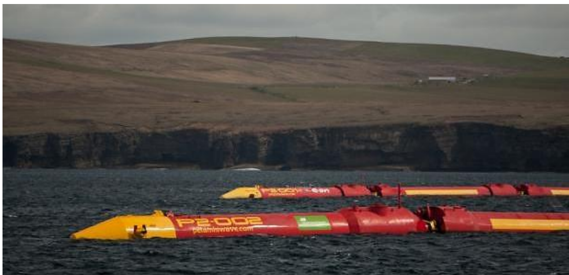
Figure 10: Illustration of Phase 5, array of two Pelamis P2 WECs undergoing trials at EMEC [53].
