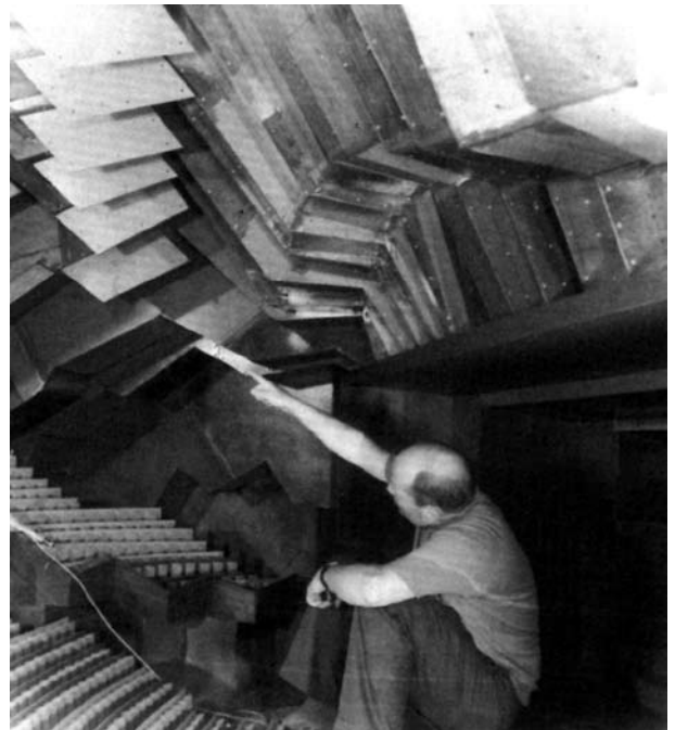
Figure 27: Vilhelm Lassen Jordan sitting in a large scale model ready for acoustic testing.
