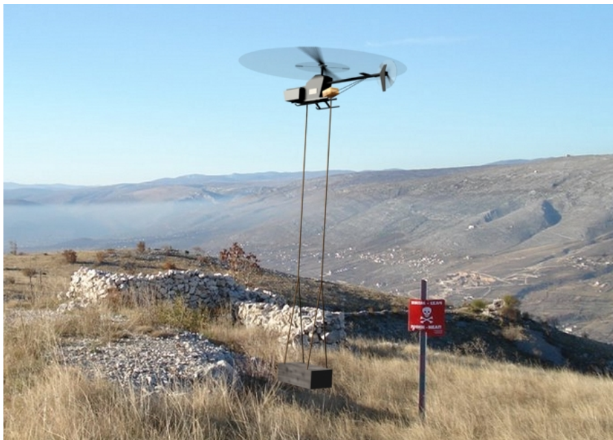
Figure 1.7: The mine detection principle with the detection equipment in the slung load close to ground.
