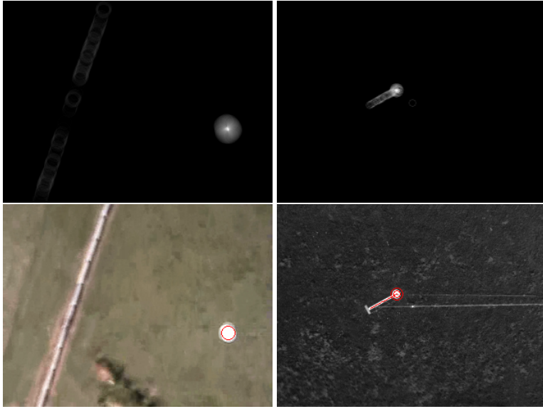
Figure 6.4: Top: Output of the Hough transform. Bottom: The output of the vision system with the located slung loads indicated by red circles.
