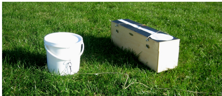
Figure 2.5: The demonstration slung loads. To the left the single wire slung load and to the right the dual wire slung load.
