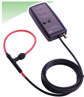
Figure 8.15: CWT current probe, to be used for the cable measurements.
