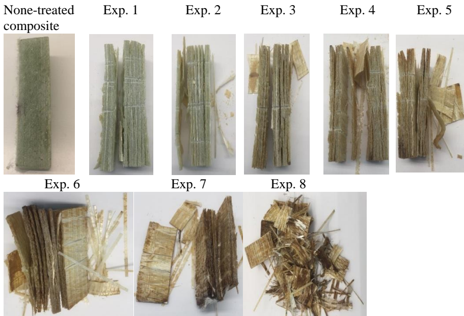
Fig. 21 Appearance of composites subjected to acetone recycled from 1 and up to 8 times.
