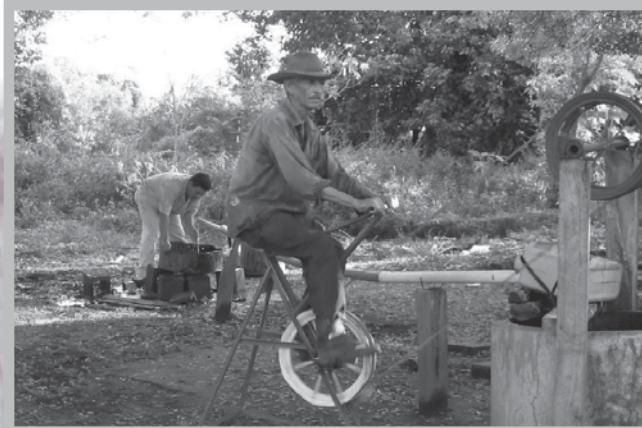
Member of APRAINORES' directive council, Manuel Enriquez, on his bicycle water pump to water cattle and irrigate new citrus trees in his cashew plantation.
