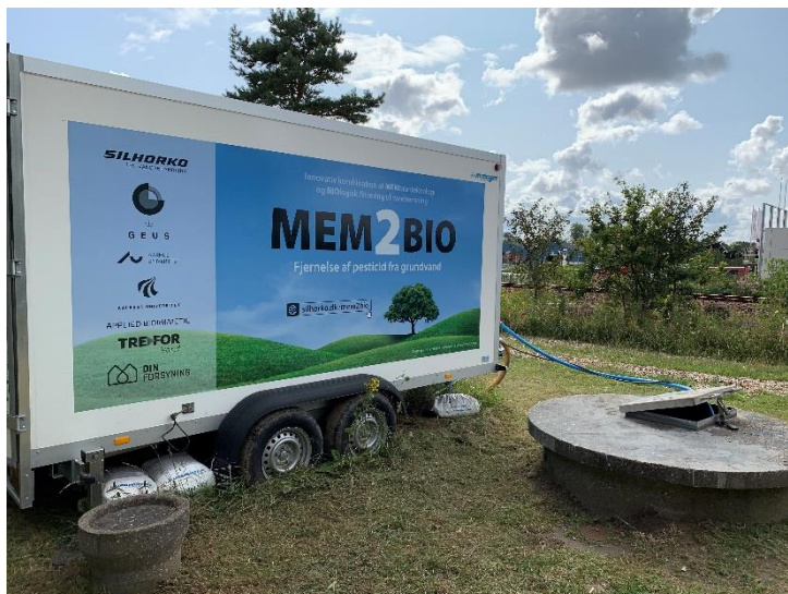
Figure 7-1 An isolated trailer containing pilot plant facilities for MEM2BIO project located by a drinking water well contaminated with BAM in Esbjerg.
