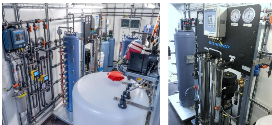
Figure 7-2 Photo showing inside of the pilot plant. The membrane train is shown on the right.
