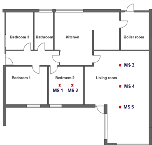
Figure 4-7. Layout of the building and the location of the measuring stands (MS 1-5) for the local thermal comfort measurements.
