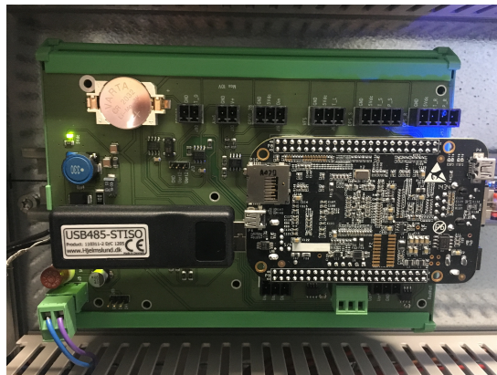
Fig. E.5: Electronics that collects the data and communicates with the cloud. Example of components are microprocessor, MODBUS and Wifi modules.
