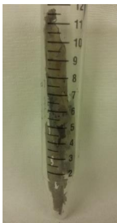
Figure 17: Unconverted plastic material collected after hydrothermal processing of LD-PE using the following conditions: 400 °C, 15min, without catalyst.
