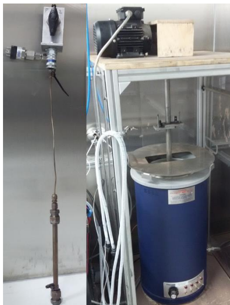
Figure 5: On the left: an example of micro-batch reactor, used for the HTL experiments. On the right: the fluidized sandbath to provide the heat for the reaction.
