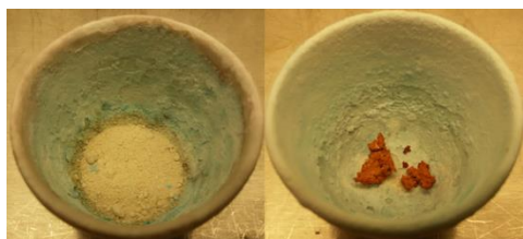
Figure 25: Ash from fish sludge (left) and from sewage sludge (right) after 3h at 775°C.
