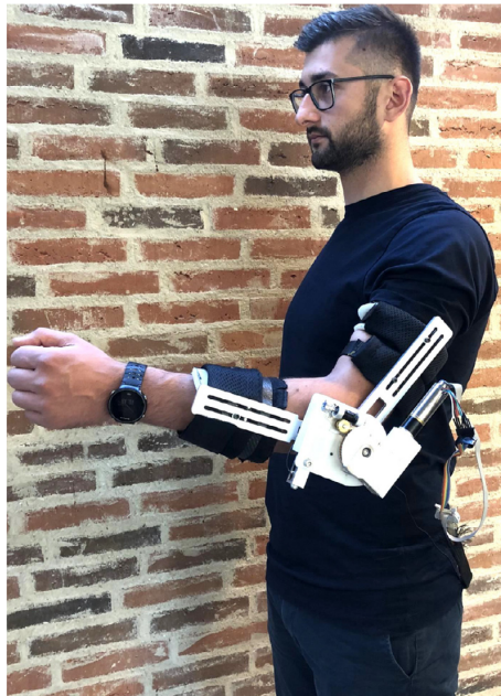
Fig. 27. Wearable elbow exoskeleton prototype mounted on the arm of a subject.
