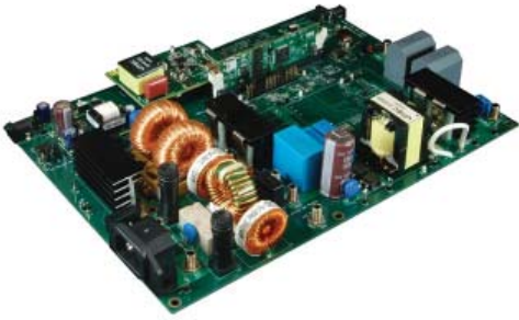
Fig. 5. Photo of TI's microinverter [21].
