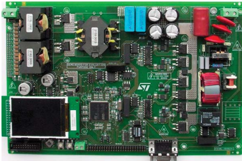
Fig. 7. Photo of the microinverter from ST Microelectronics [15].
