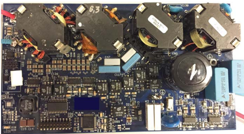
Fig. 9. Photo of the impedance-source-based PV microinverter topology [24].
