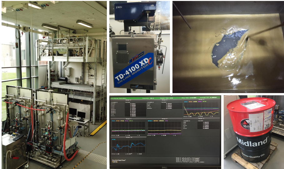
Fig. 3.1: Photos of the pilot-plant. Left: the pilot-plant; top middle: two of the three online monitor types on a movable skid; bottom middle: the Matlab Simulink Real-Time interface of the pilot-plant; top right: example of the OiW mixture in the buffer tank; bottom right: barrel of the Midland non-detergent Society of Automotive Engineers (SAE) 30 oil used.
