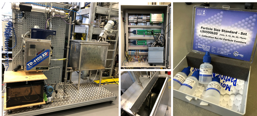
Fig. 4.1: Photos of the skid-mounted test setup. Left: the test setup for testing different online quality monitors; top middle: electrical control panel; bottom middle: the supply tank with a mounted mixer; right: calibration particles manufactured by BS-Partikel.
