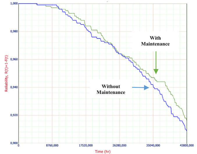
Fig. 7. Reliability of power conditioner without repair and inspection (blue) and with repair and inspection (green) considering Weibull distribution. (For interpretation of the references to colour in this figure legend, the reader is referred to the web version of this article.)
