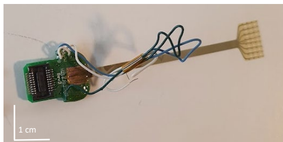
Figure 3.1. 32-channel Neuronex \mu ECoG used for recording from S1.
