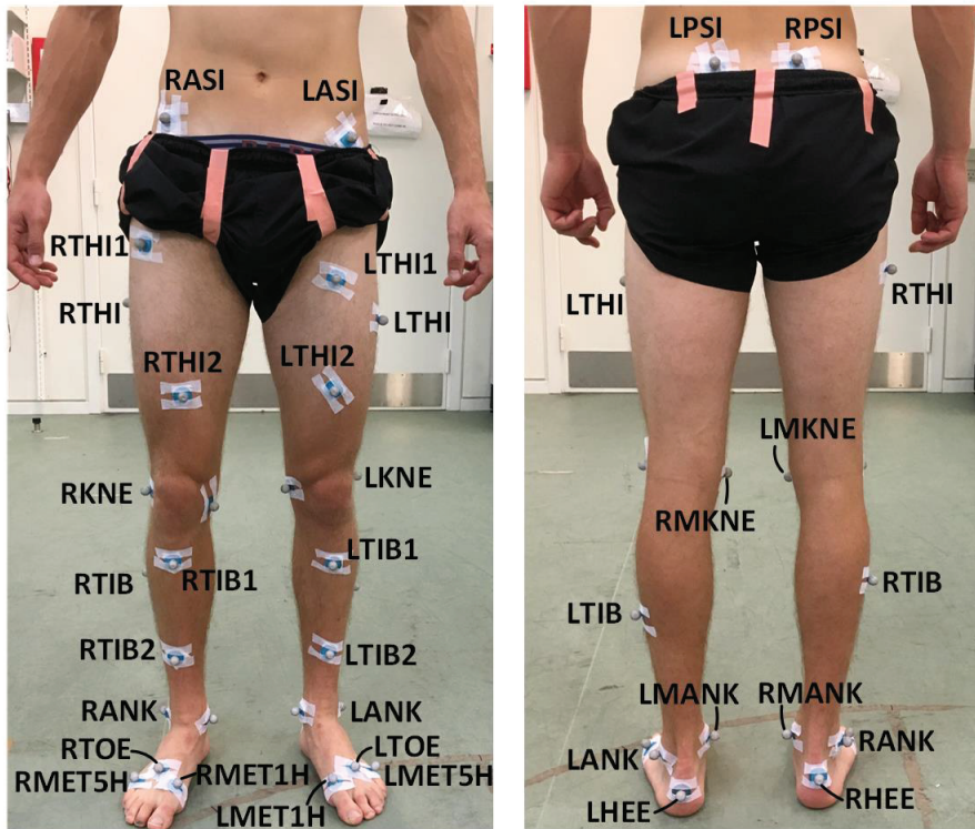
Figure 1. The marker placements used to obtain initial kinematics for brace development.
