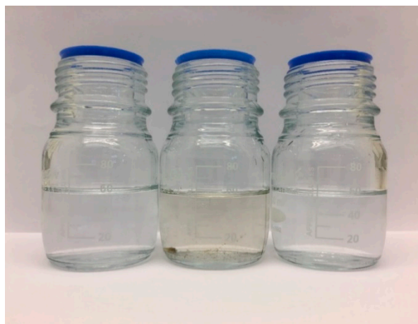
Figure 7. Samples of wastewater treatment plant effluent ( middle ), permeate of the membrane with surfactant/oxide ratio (S/O) = 0.5 ( left ), and permeate of the membrane with S/O = 2.0 ( right ).
